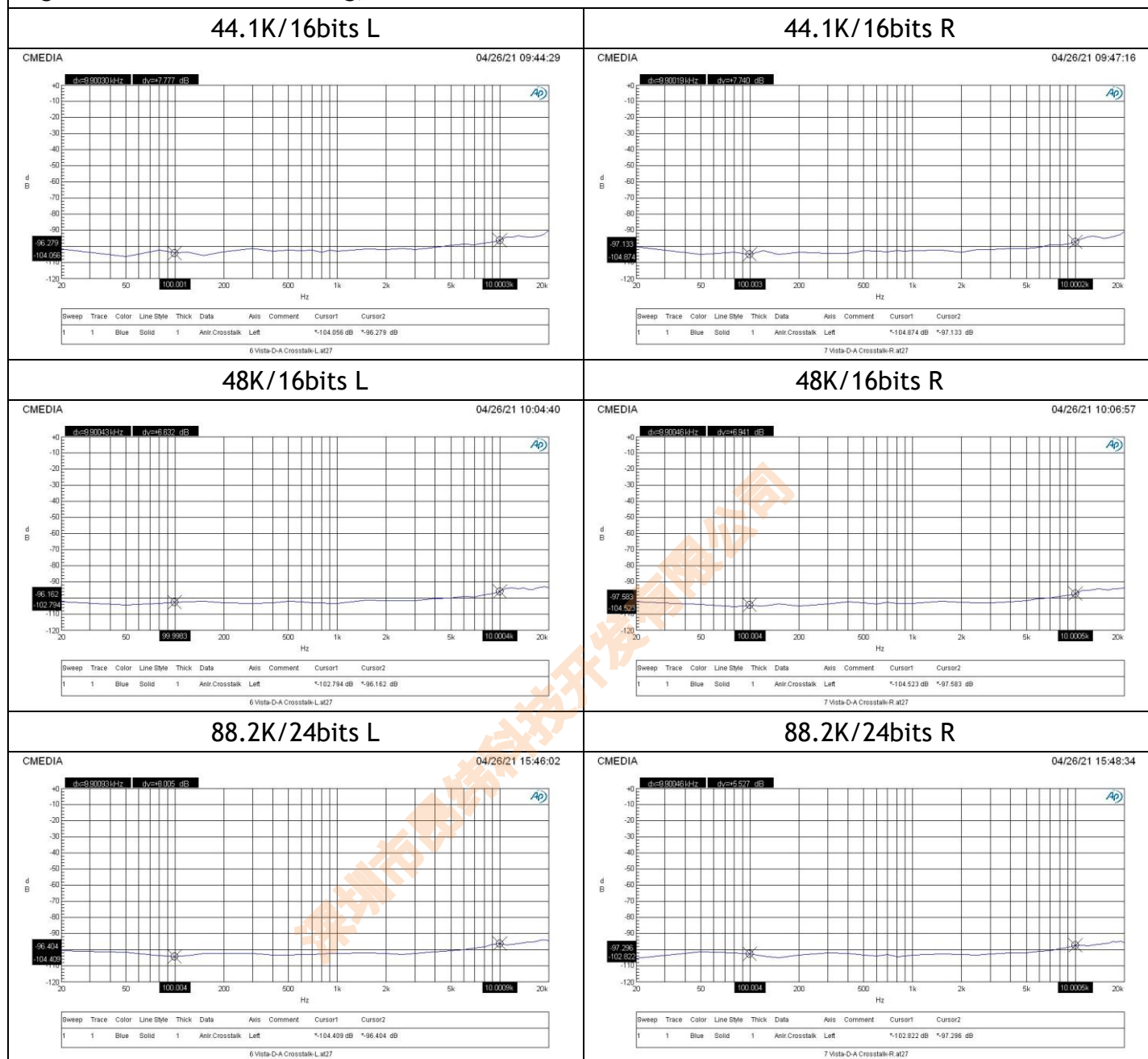
Figure 7 : DAC 10K \Omega loading, Cross-talk
