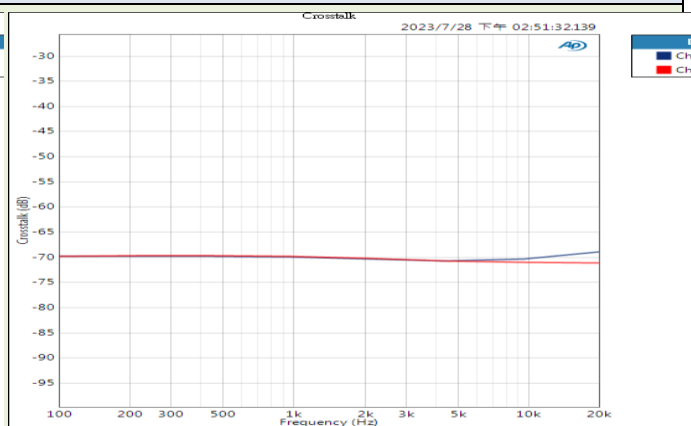
Cross-talk @ 32Ω with 33Ω cascade loading
