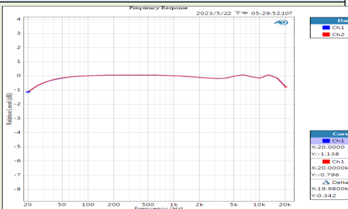
Frequency Response 20dB Gain Figure 15
